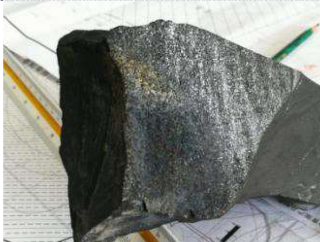
Figure 3: A sample of tectonic-coal in Qianjing Coal Mine
