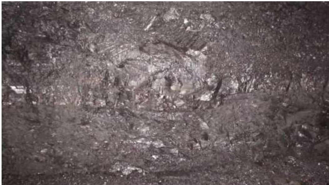
Figure 8: Tectonic coal seen at the reverse fault of the No.8303 working face in Wangping.
